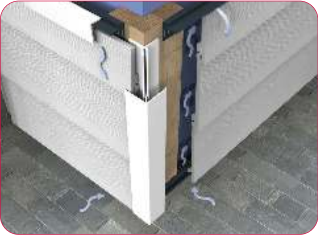
It is essential that continuous ventilation is maintained between the vertical battens from top to bottom and adequate expansion is allowed for at the ends of the boards.
